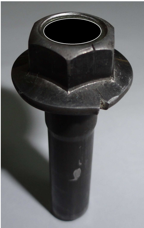
Figure 6: Cracks on a screw
